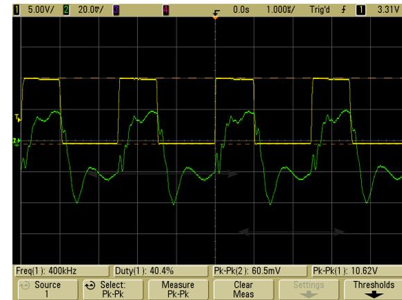
Figure 4.9. Measured waveforms with input filter inductors bypassed
