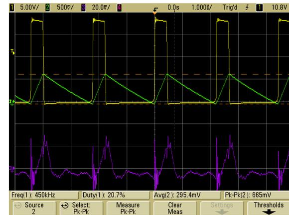
**Figure 5.14.** Measured TPS54160 regulator waveforms with inductor L6 at:  $V_{in} = 18 \text{ V}$ ,  $I_{out} = 0.3 \text{ A}$  and  $f_{sw} = 450 \text{ kHz}$
